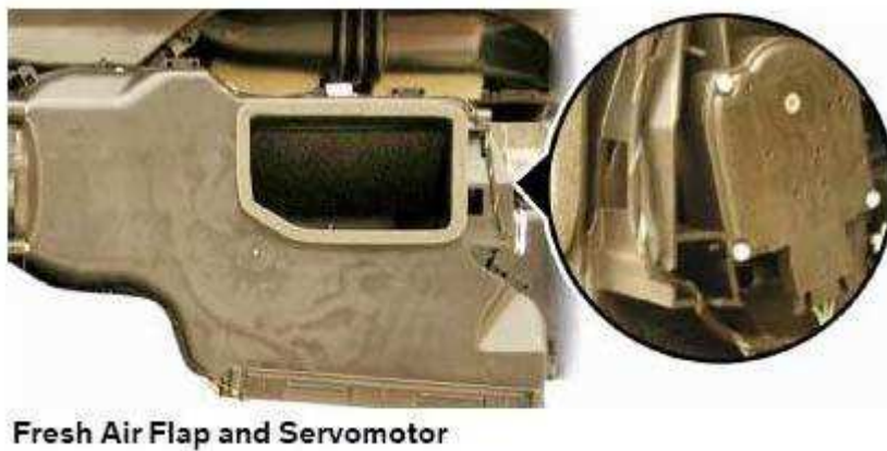
Fig. 24: Fresh Air Flap And Servomotor Courtesy of BMW OF NORTH AMERICA, INC.
