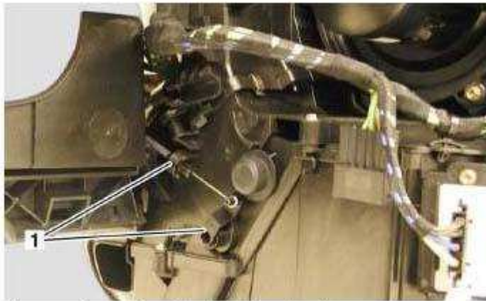
Fig. 25: Temperature Flap Control Mechanism And Flap Control Cable Connection Courtesy of BMW OF NORTH AMERICA, INC.
