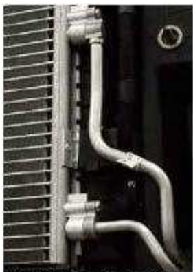
A/C Lines at Condenser
