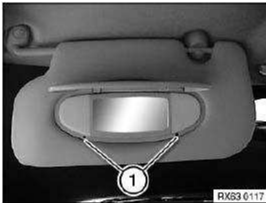
Fig. 70: Identifying Mirror Clip Points Courtesy of BMW OF NORTH AMERICA, INC.
