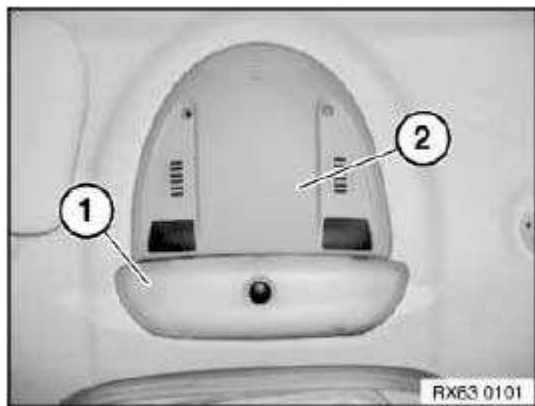
Fig. 40: Identifying Trim Roof Operating Unit Courtesy of BMW OF NORTH AMERICA, INC.
