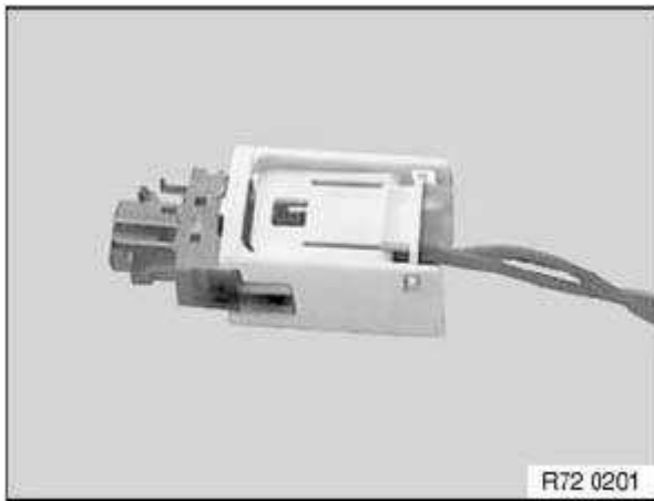
Fig. 22: Identifying Airbag Plug Connection Courtesy of BMW OF NORTH AMERICA, INC.
